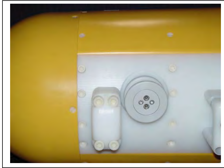
Figure 4-3: Cable Retainer and Guide Wheel
