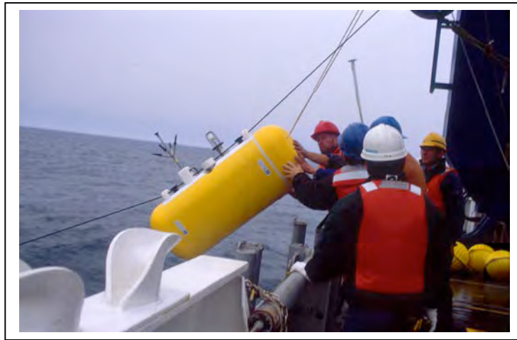
Figure 7-13: Recovering an MMP
