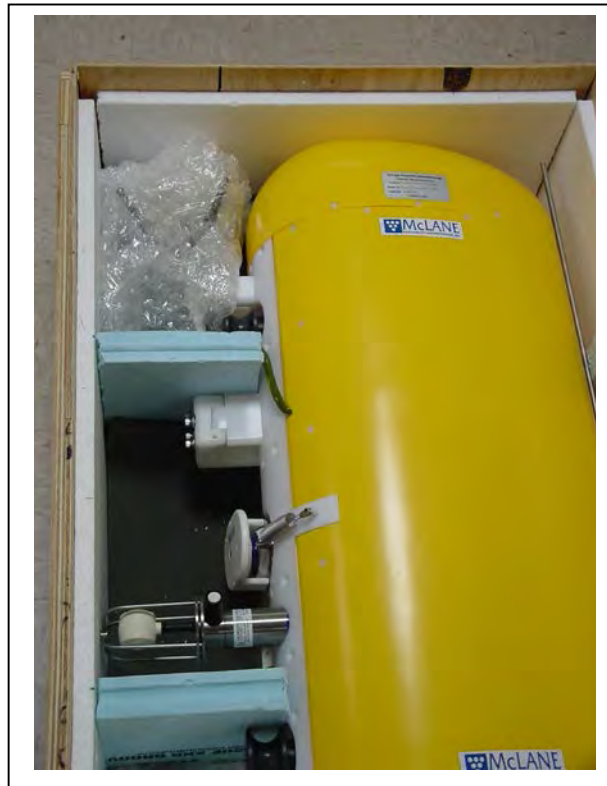
Figure 8-2: Fitting the MMP in the Crate
