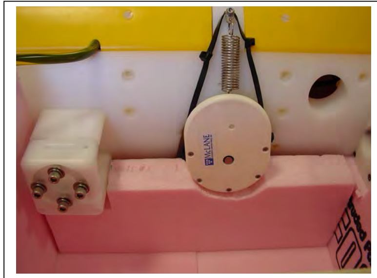
Figure 8-3: Stabilizing the Motor in the Crate
