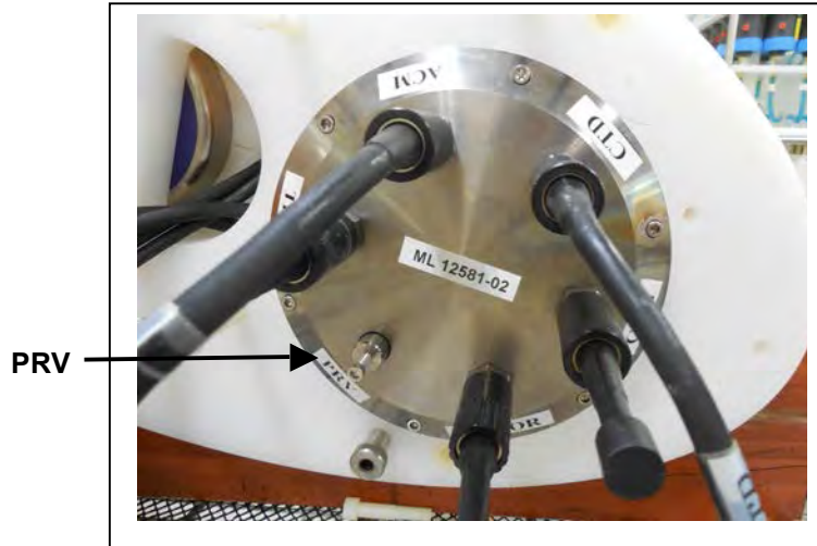
Figure 4-9: Controller End Cap, with PRV
