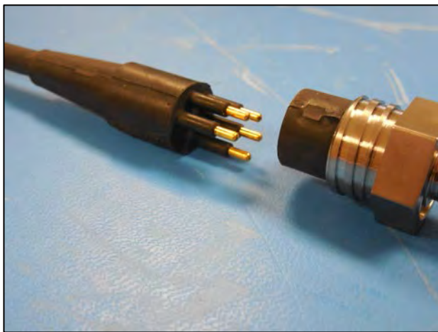
Figure 5-26: 5-Pin and 3-Pin connectors
