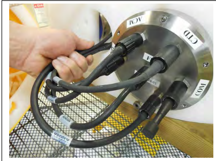
Figure 4-6: Gathering Excess Cable Length
