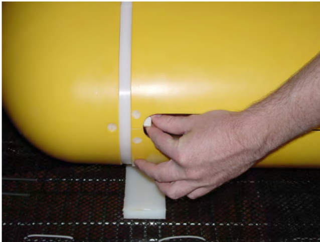
Figure 4-5: Unscrewing the Nylon Cap Screw and Removing End Cap
