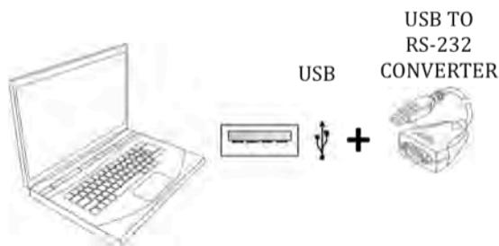
Figure 2-2: Computer COM Setup Styles
