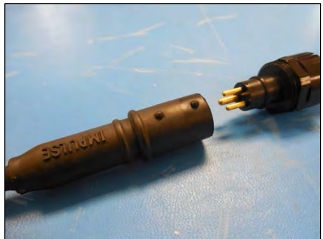
Figure 5-26: 5-Pin and 3-Pin connectors
