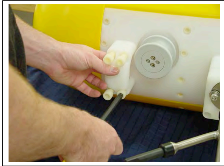
Figure 7-3: Removing the Cable Retainers
